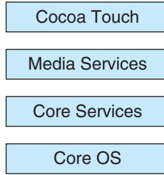
Figure 2.17 Architecture of Apple's iOS.
