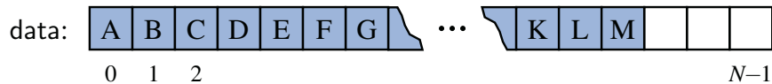
Figure 6.5: Using an array to store elements of a queue, such that the first element inserted, “A”, is at cell 0, the second element inserted, “B”, at cell 1, and so on.
