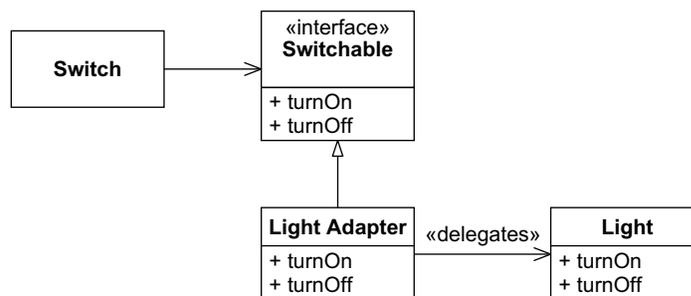
Figure 25-4 Solving the Table Lamp with ADAPTER
