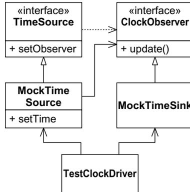
Figure 24-5 Removing ClockDriver and TimeSink
