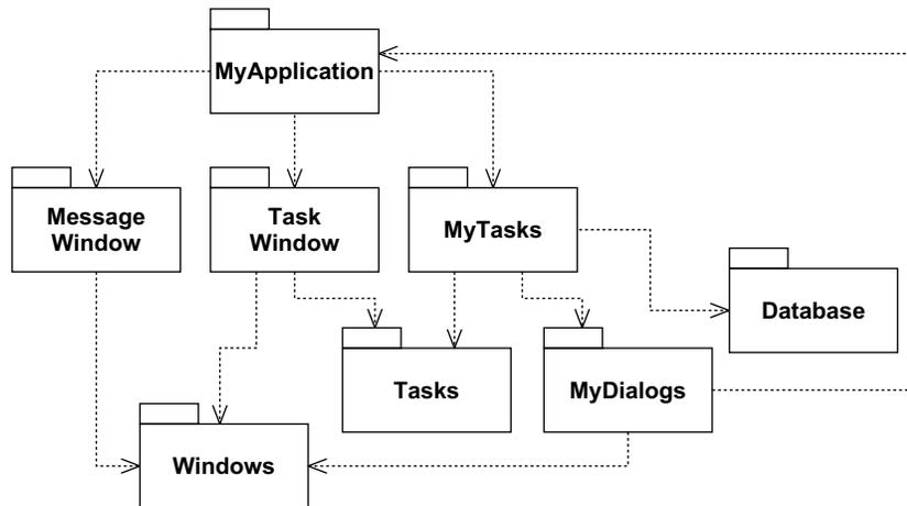
Figure 20-2 A Package Diagram with a Cycle
