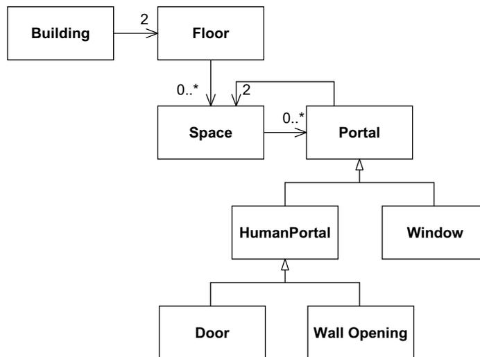
Figure 30-4 Floor Plan Data Structure
