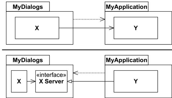
Figure 20-3 Breaking the cycle with dependency inversion
