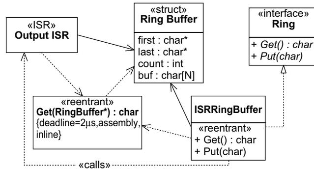
Figure B-5 Output Interrupt Service Routine
