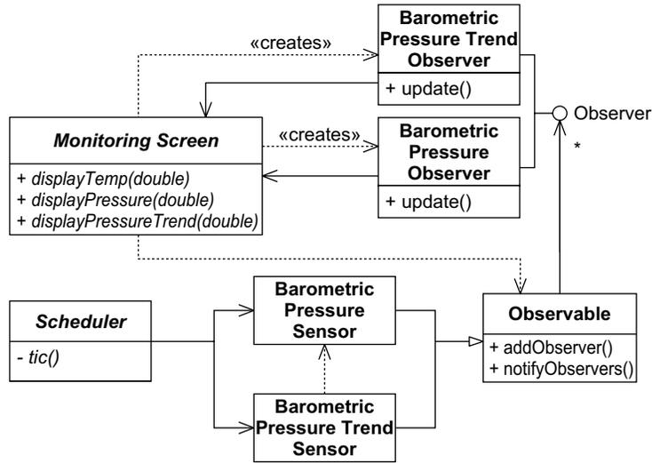
Figure 27-6 Barometric Pressure Observers
