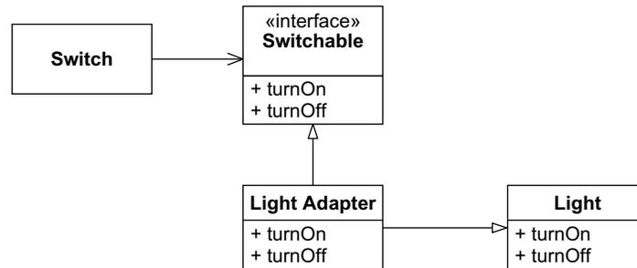
Figure 25-5 Solving the Table Lamp with ADAPTER
