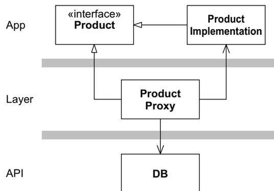
**Figure 26-8** How the PROXY inverts the dependency between the application and the Layer
