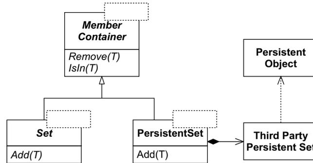
Figure 10-4 A solution that is LSP compliant
