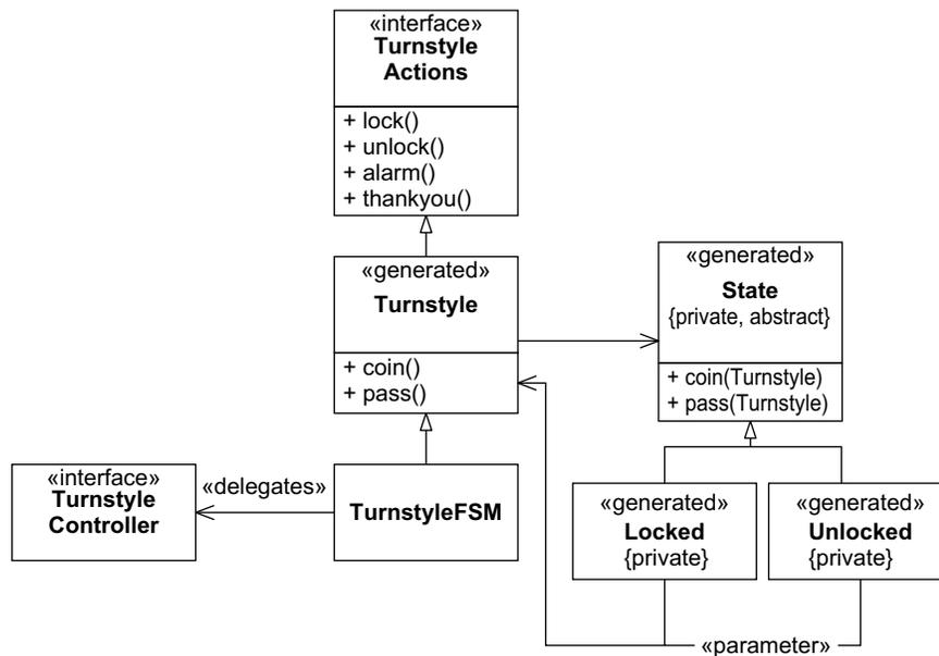
**Figure 29-5** Three-Level FSM
