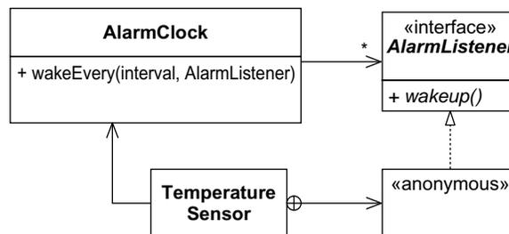
Figure 27-7 Decoupled Alarm clock
