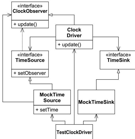
Figure 24-4 Breaking the dependency of TimeSource upon ClockDriver
