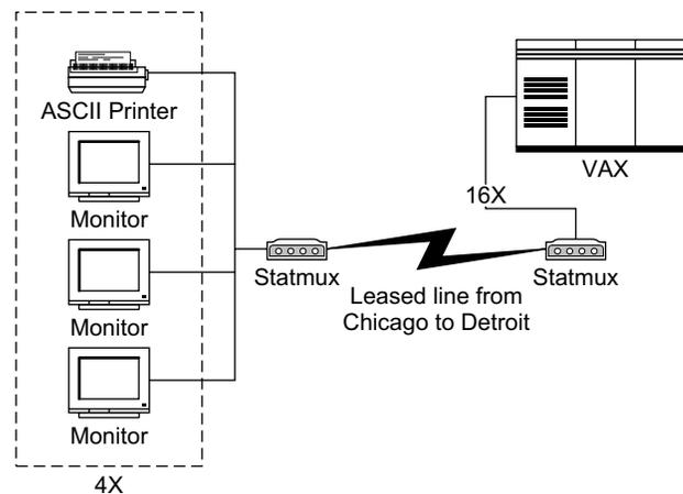
**Figure B-1** Typical Statistical Multiplexor Application
