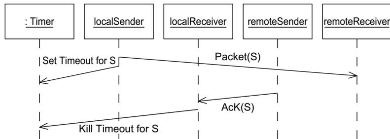
**Figure B-10** Acknowledgment of a packet: Normal
