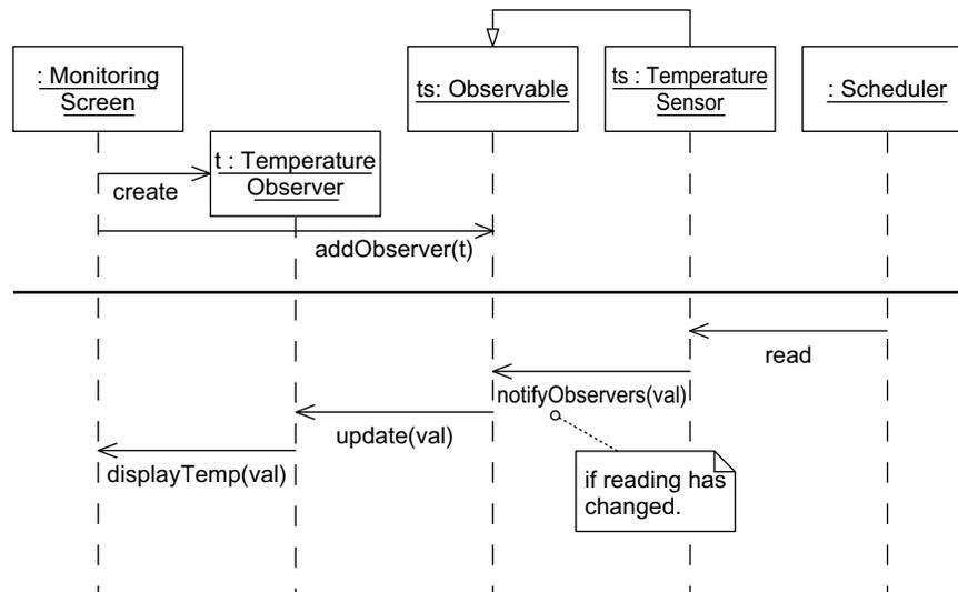
Figure 27-5 Decoupled UI sequence diagram
