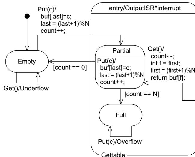
Figure B-6 Output Service Interrupt State machine
