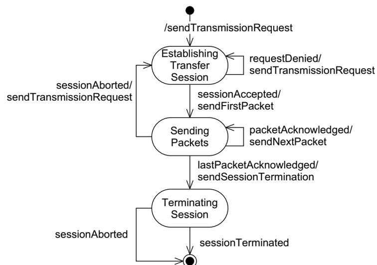
Figure 29-7 Sending large block using many packets
