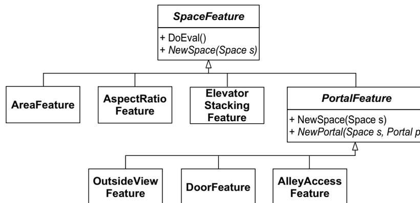
**Figure 30-5** TEMPLATE METHOD structure of the scoring features
