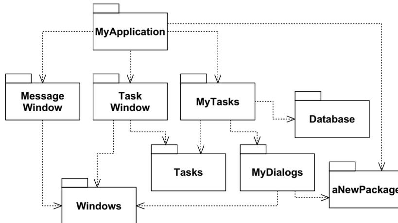
Figure 20-4 Breaking the cycle with a new package
