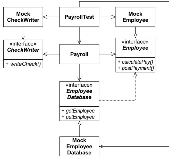
Figure 4-2 Decoupled Payroll using Mock Objects for testing
