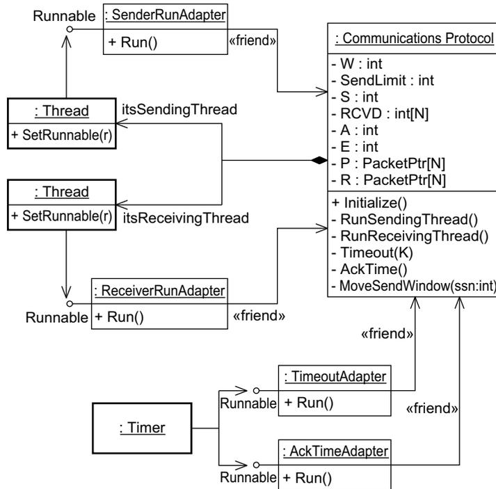
Figure B-8 Object Diagram: Just after protocol object has been initialized
