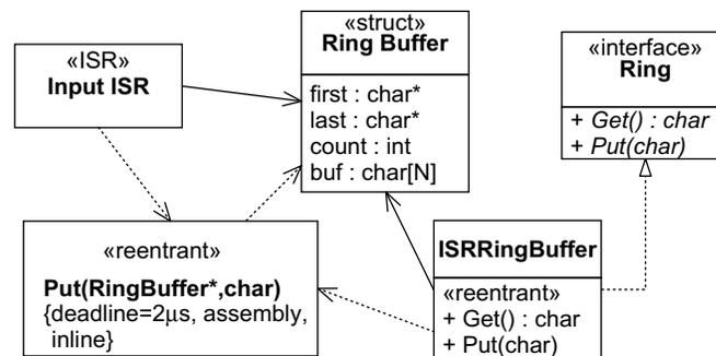
Figure B-3 The Input Service Interrupt Routine
