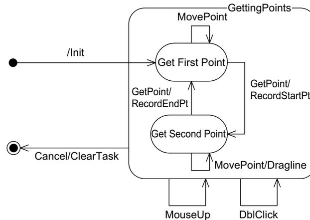
**Figure 30-11** Finite-State Machine for the Measure Task.
