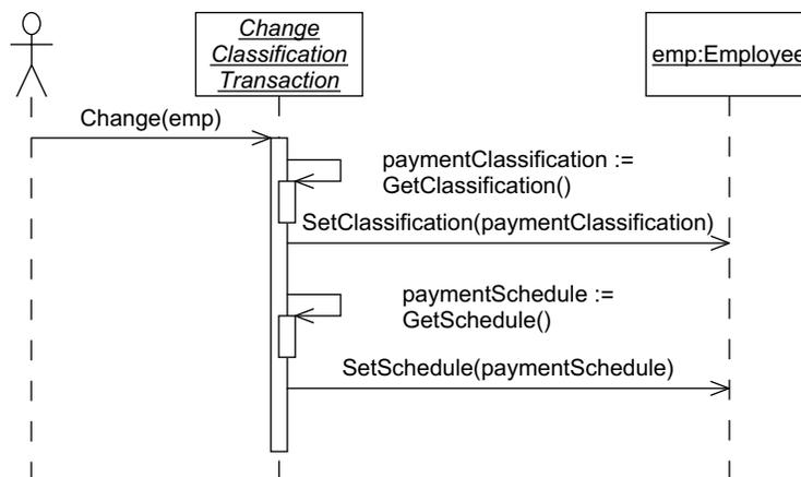
Figure 19-18 Dynamic Model of the `ChangeClassificationTransaction`
