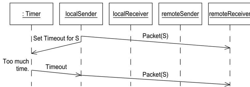
**Figure B-11** Acknowledgment lost: Retransmission
