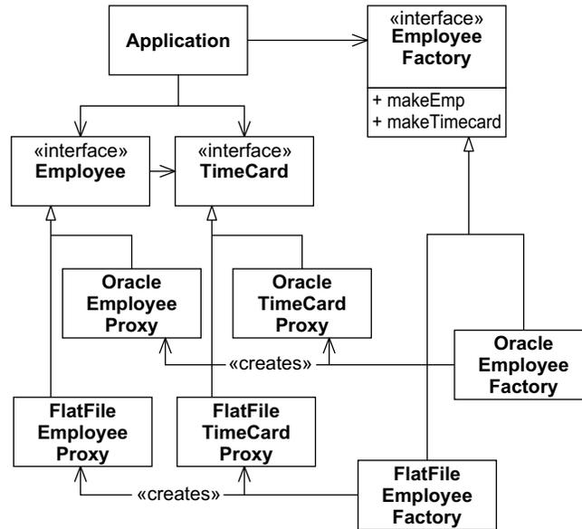
Figure 21-3 Substitutable Factory
