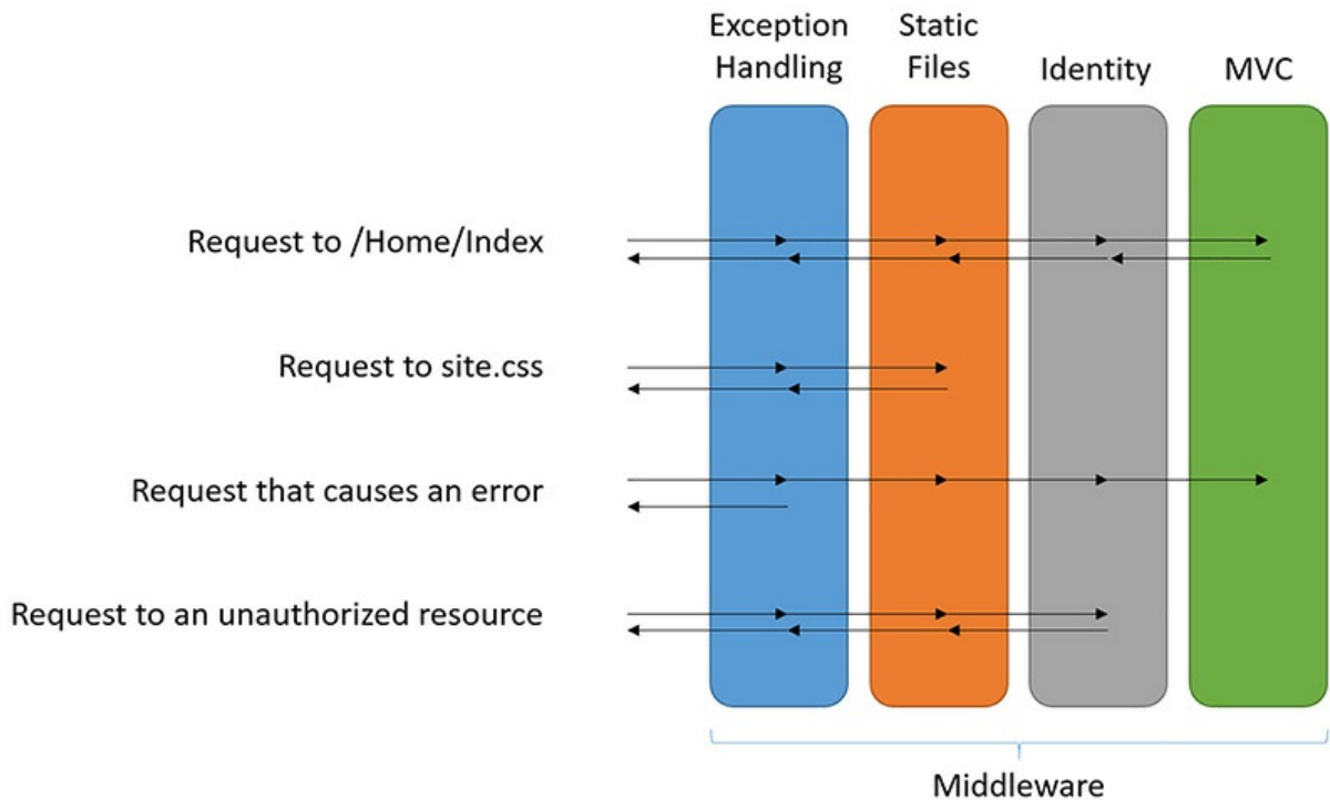
FIGURE 3-3 An illustration showing examples of different request types as handled by middleware
