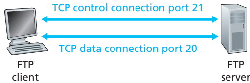
Figure 2.15 ♦ Control and data connections
