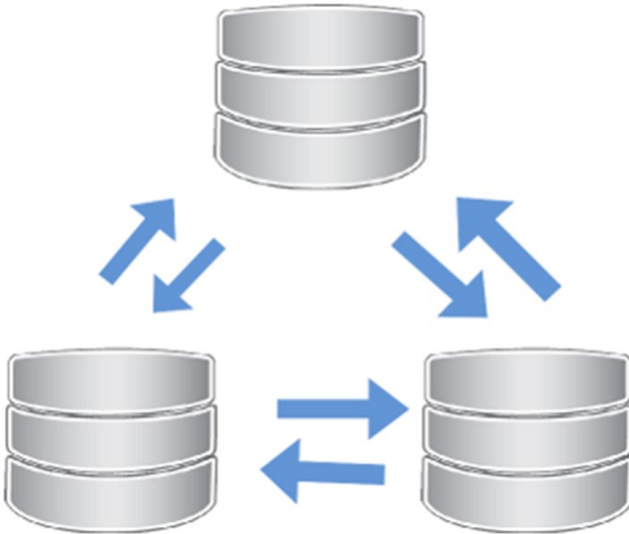
Figure 5-3. Multimaster replication topology
