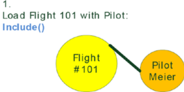
Figure 9-1. Loading strategies in the Entity Framework 1.0 to 6.x. Entity Framework Core currently supports only three strategies; lazy loading is missing.
