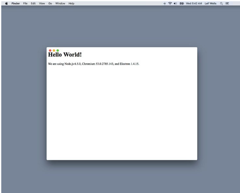
Figure 4-10. The Electron application in a frameless window with window controls added in the inset mode
