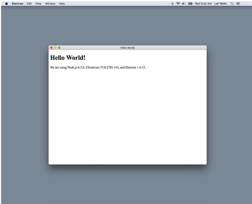
Figure 4-2. The starter Electron window opening using the ‘ready-to-show’ event
