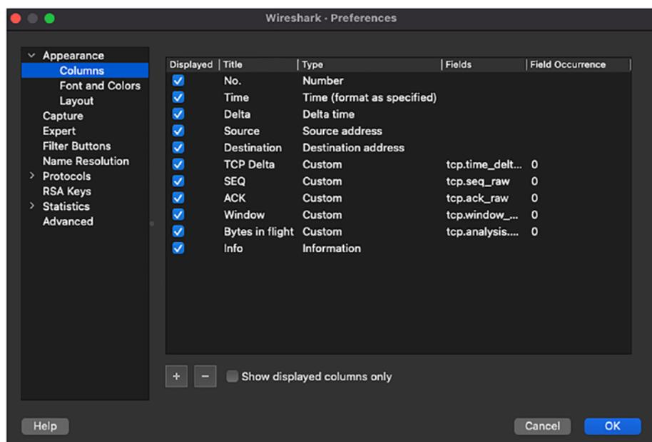
**Figure 4-36.** Custom columns for TCP profile
