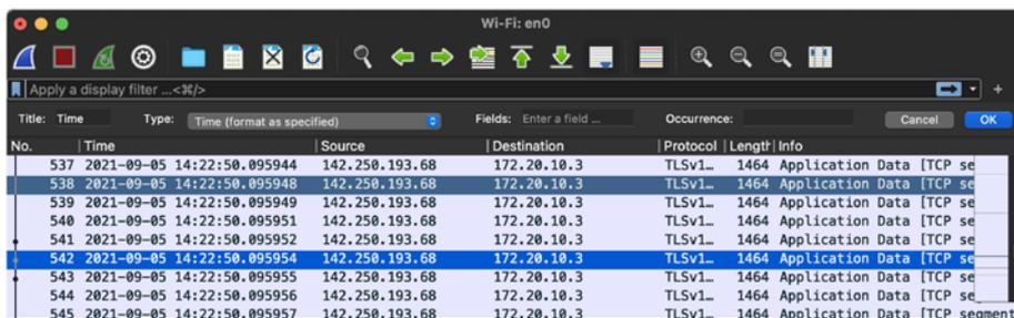
Figure 2-21. Wireshark with UTC date and time timestamps
