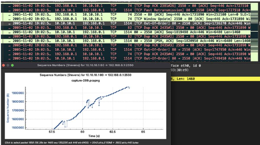
*Figure 4-20. TCP retransmissions and OOO packets in Stevens graph*
