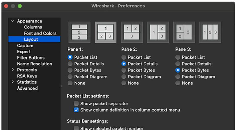
*Figure 2-2. Custom Wireshark layout*
