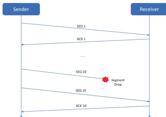
**Figure 4-14.** TCP retransmission
