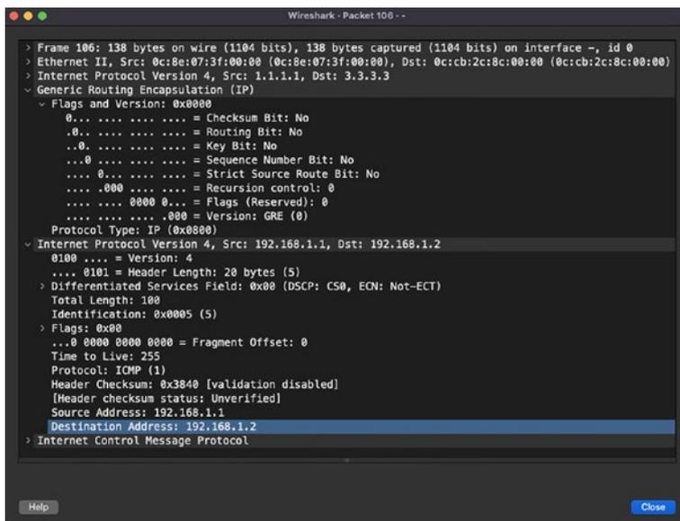
**Figure 5-25.** GRE encapsulation
