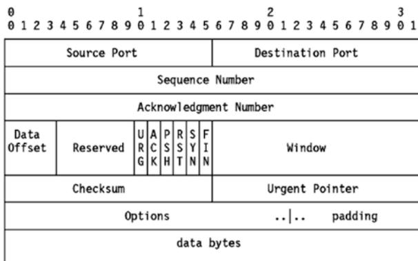
**Figure 4-3.** TCP header
