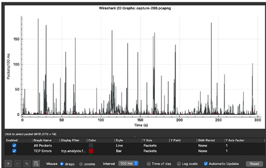
*Figure 4-32. Microbursts in I/O graphs*
