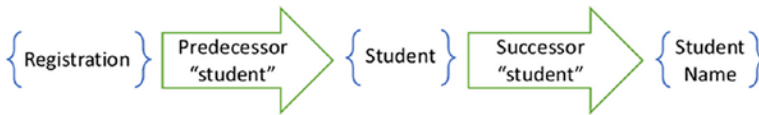
Figure 10-3. Finding the name of a registered student involves stepping up to the student and then down to the name
