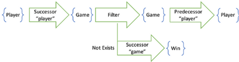
Figure 9-25. A pipeline for finding current opponents takes an additional predecessor step to the player
