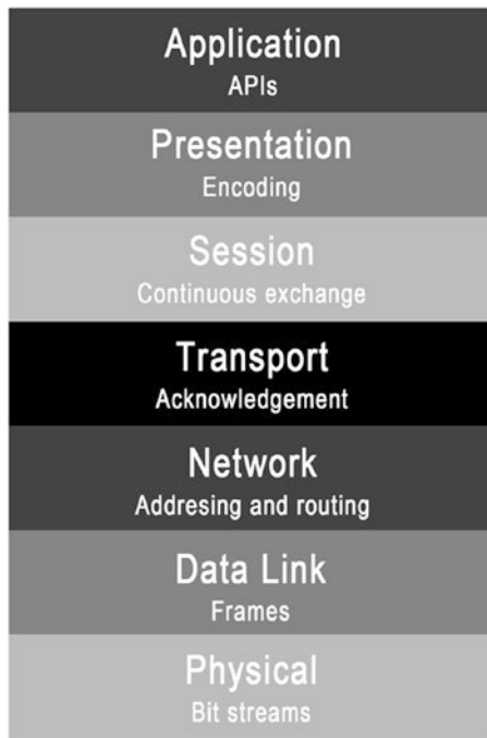
Figure 11-1. The OSI model of network communication divides protocols into seven layers of abstraction
