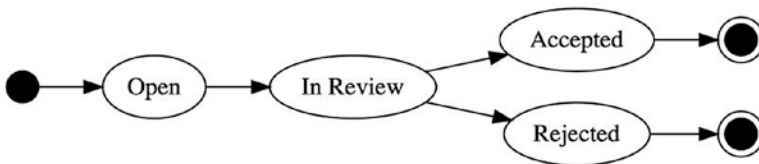
Figure 6-7. The state transition diagram of a commit, as implemented in a separate tool
