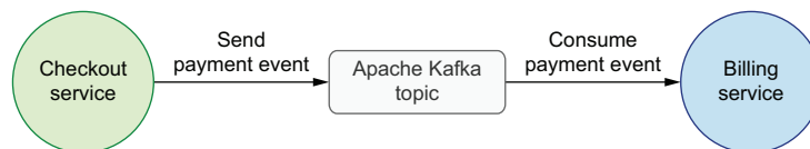
Figure 11.15 Billing and checkout service that work as event-based processes
