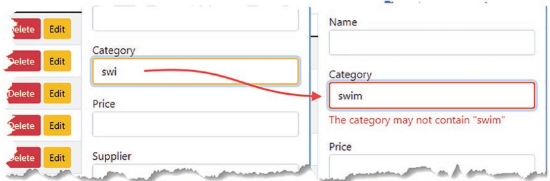
Figure 22-11. Using an asynchronous validator
