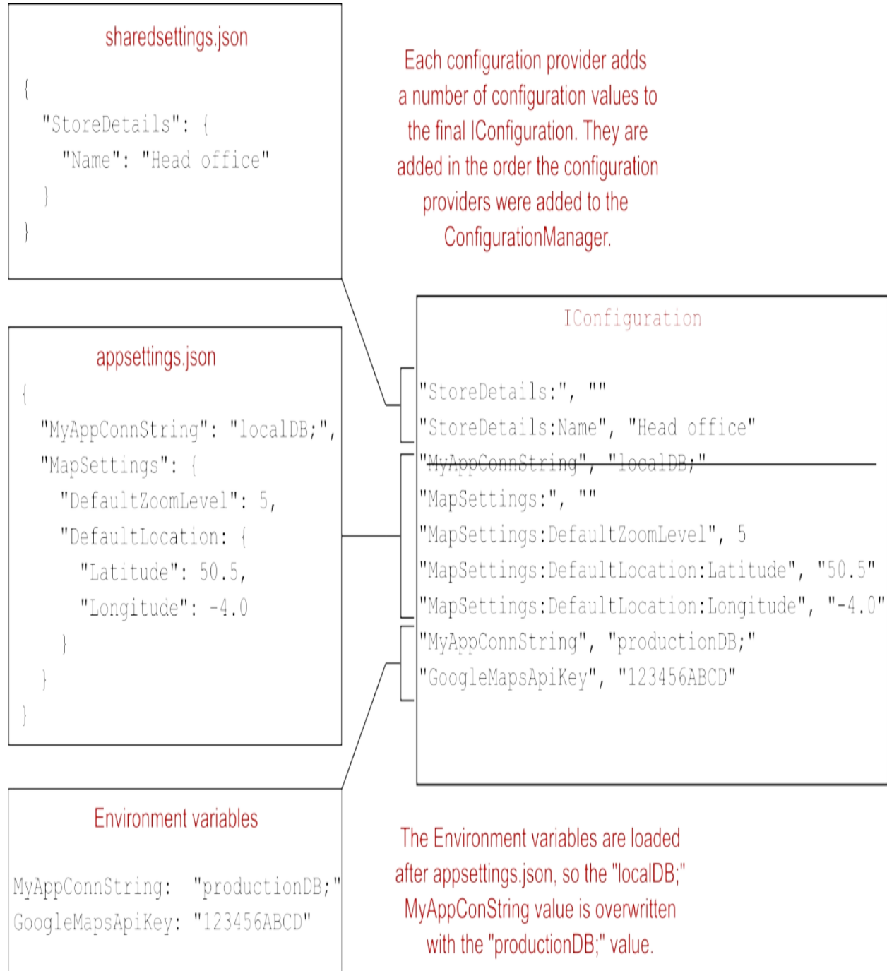
Figure 10.4 The final IConfiguration includes the values from each of the providers. Both appsettings.json and the environment variables include the MyAppConnString key. As the environment variables are added later, that configuration value is used.
