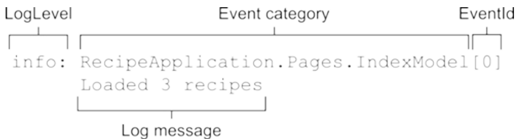
Figure 26.4 An example log message as it's written to the default console provider. The log-level category provides information about how important the message is and where it was generated. The EventId provides a way to identify similar log messages.
