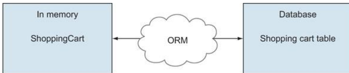
Figure 11.1. The active record pattern relies on mapping an in-memory object into an object in a data store that mutations are then saved to.
