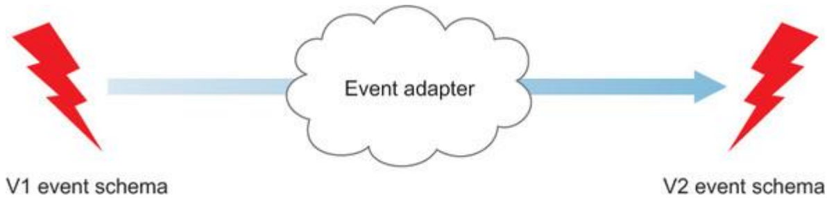
Figure 11.5. Event adapters allow you to modify events from a journal to an actor and vice versa, enabling you to make changes to event-sourced applications while also maintaining the full event history.
