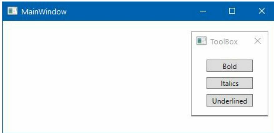
7. Drag the ToolBox window and you can see that you are able to move it outside the MainWindow. Now perform some operations, such as minimizing and closing, on the MainWindow, and you will see that the ToolBox window also acts according to its owner.
