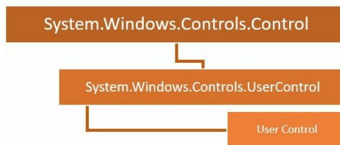
Generally, the User Control gets placed inside a XAML page with tight bonding to its code behind. You can directly access its UI elements from the code behind and do some specific operations.
