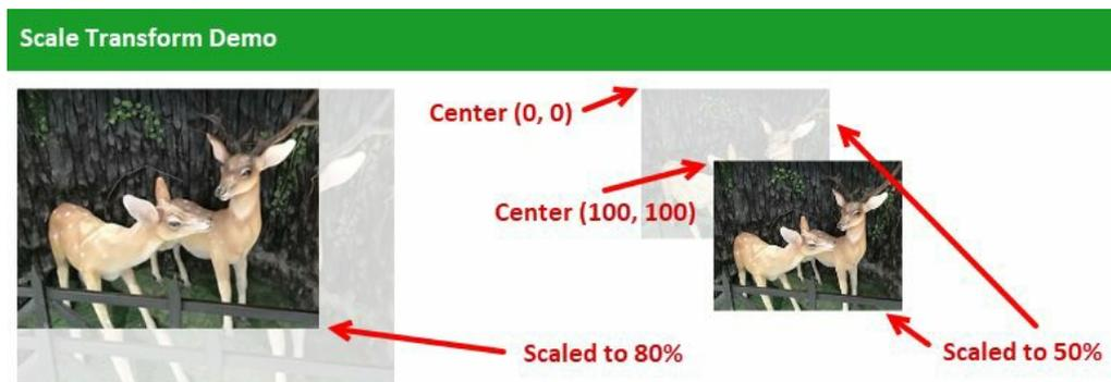
For the third and fourth images, both are scaled to 50%. But, as you see on the UI, the positions of the said images are different. The properties `centerX` and `centerY` are used to set the scaling center position. The third image has the scaling center set at (0,0), whereas the fourth one has its center position set at (100,100):
