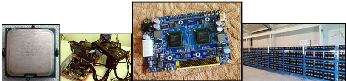
Four types of mining (CPU, GPU, FPGA, and ASIC)
