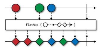
The marble diagram touches on an important aspect of flatMap(). Each upstream event (circle) is turned into an Observable of two diamonds separated by some delay.
