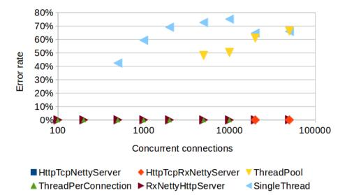
Errors, as reported by the wrk load test tool are nonexistent to marginal for all of the implementations except SingleThread and ThreadPool. This is an interesting tradeoff: ThreadPool always responds as soon as possible, much faster than competitors. However, it is also very eager to reject requests immediately when it is being overwhelmed. Of course, you can implement a similar mechanism on top of a reactive implementation with Netty/RxJava.
