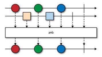
The sample that follows illustrates how amb() works with two streams. Pay attention to initialDelay parameter that controls which Observable starts emitting first:
