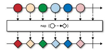
The map() operator takes a function that can change the shape of input event from circle to square. This transformation is applied to each item flowing through it.
