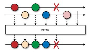
The merge() operator is used extensively when you want to treat multiple sources of events of the same type as a single source.<sup>4</sup> Also, if you have just two Observables you want to merge(), you can use obs1.mergeWith(obs2) instance method.
