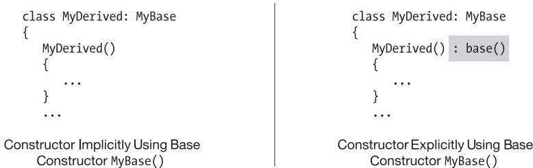
Figure 8-12. Equivalent forms of a constructor
