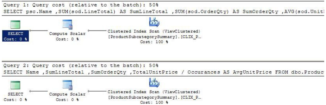
Figure 8-53. Execution plan for Indexed View pattern
