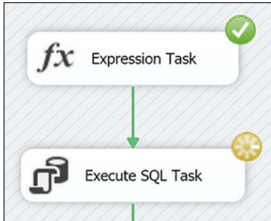
FIGURE 2-81 Execution Status in Debug Mode—Successful and In-Progress
