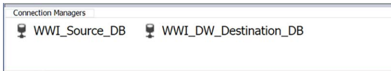
FIGURE 2-17 Renamed OLE DB Connection in Connection Manager
