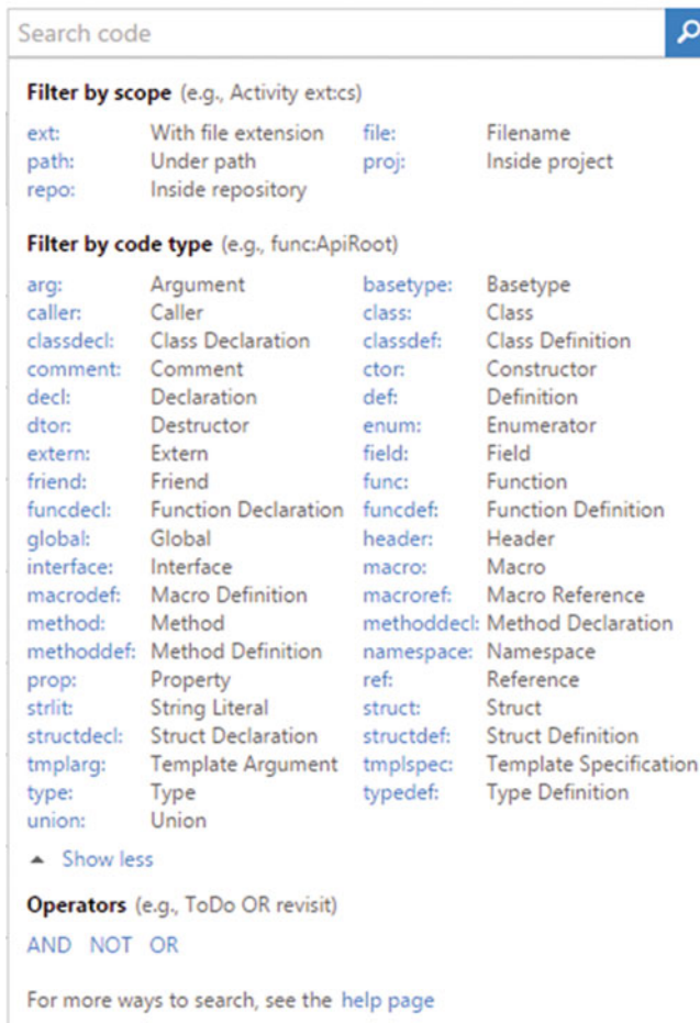
Figure 6-21. Available filters when searching through code
