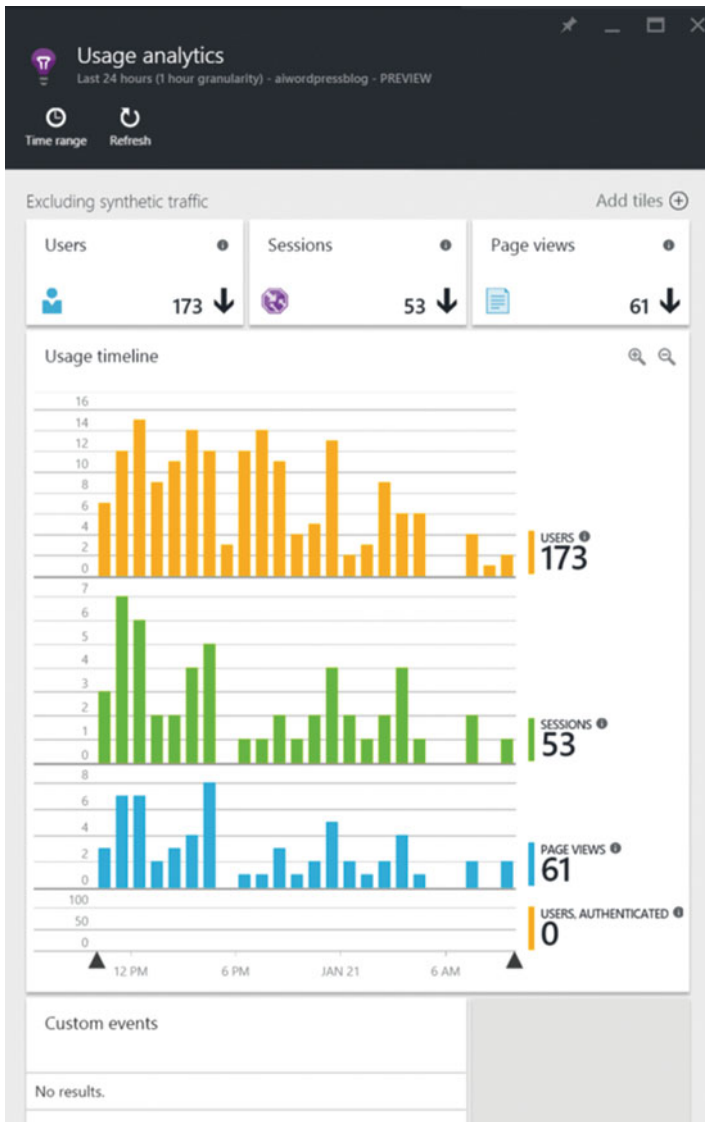
Figure 13-11. Application Insights can track usage telemetry
