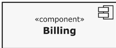
Figure A-9. The UML notation for a component
